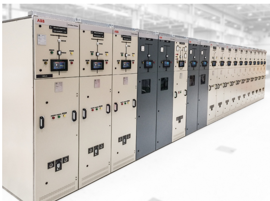
One of the eight new 825 V DC switching gear of the second line of the Warsaw Metro. It has been equipped with CZAT7 automation, which uses the IEC 61850 communication protocol for the needs of the Warsaw Metro.
